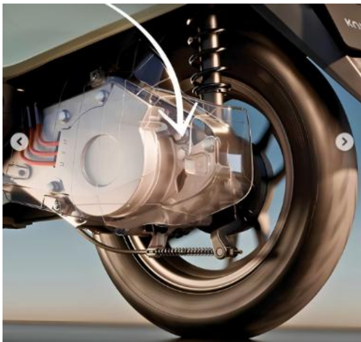
Exhibit 2: Konarc features a silent direct transmission with a swing arm mounted motor
