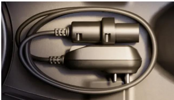
Exhibit 4: Konarc is also equipped with 450W onboard charger..
